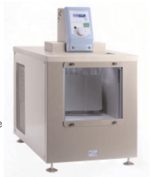
The cover of the bath has four, round, 51 mm holes with lids, for suspending glass capillary viscometers in holders. A permanent light is located in the top plate ensuring optimal visibility. The TV12LT requires only 15 liters of bath medium. A bath overflow outlet protects against expanding bath fluid. The bath can be emptied via a NEW built-in drain. A LED fluid level indicator alarms when fluid level is too low. The bath is fitted with adjustable feet for leveling.
